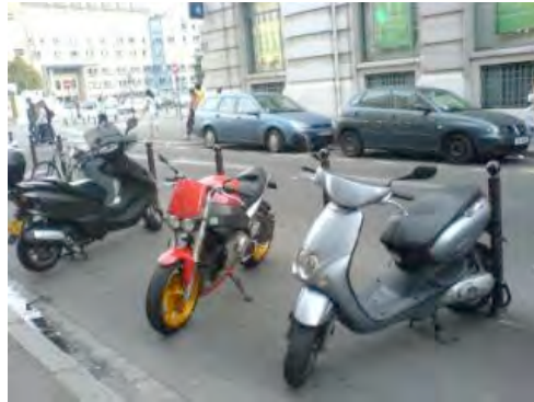
This parking bay features spaces for bicycles (left) with U-shaped "Sheffield" parking stands, and spaces for PTWs (above) with vertical posts as anchor points.
