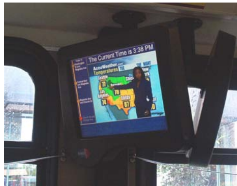
EXHIBIT 4-131 On-Board Passenger Information Display - Mounting and Screen Detail (Orlando)
