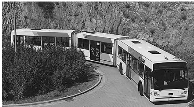
Photo 6-F. Conventional low-floor bus—24-meter (80-foot), double articulated, low-floor.
