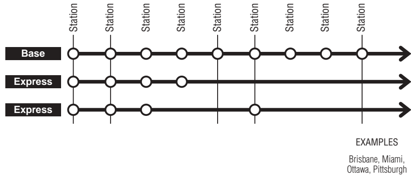
Figure 8-4. All-stop service and express BRT service overlay.
