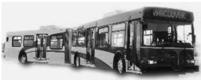
Photo 6-E. New Flyer conventional low-floor bus—18-meter (60-foot) low-floor articulated bus (Vancouver 98 B-line).
