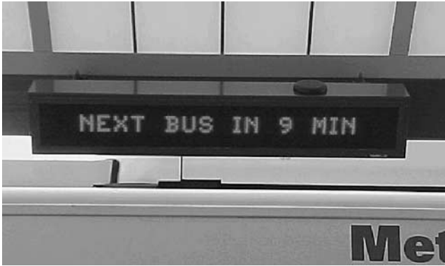
Photo 7-B. Off-board passenger information, Metro Rapid, Los Angeles.
