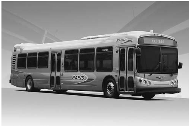
Photo 6-D. Composite 13.8-meter (45-foot) low-floor bus.
