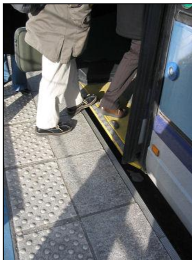
Photo 21: TEOR's guidance systems ensures that horizontal and vertical gaps between the platform and the bus are less than 5 cm for the main doors (source: Certu)
