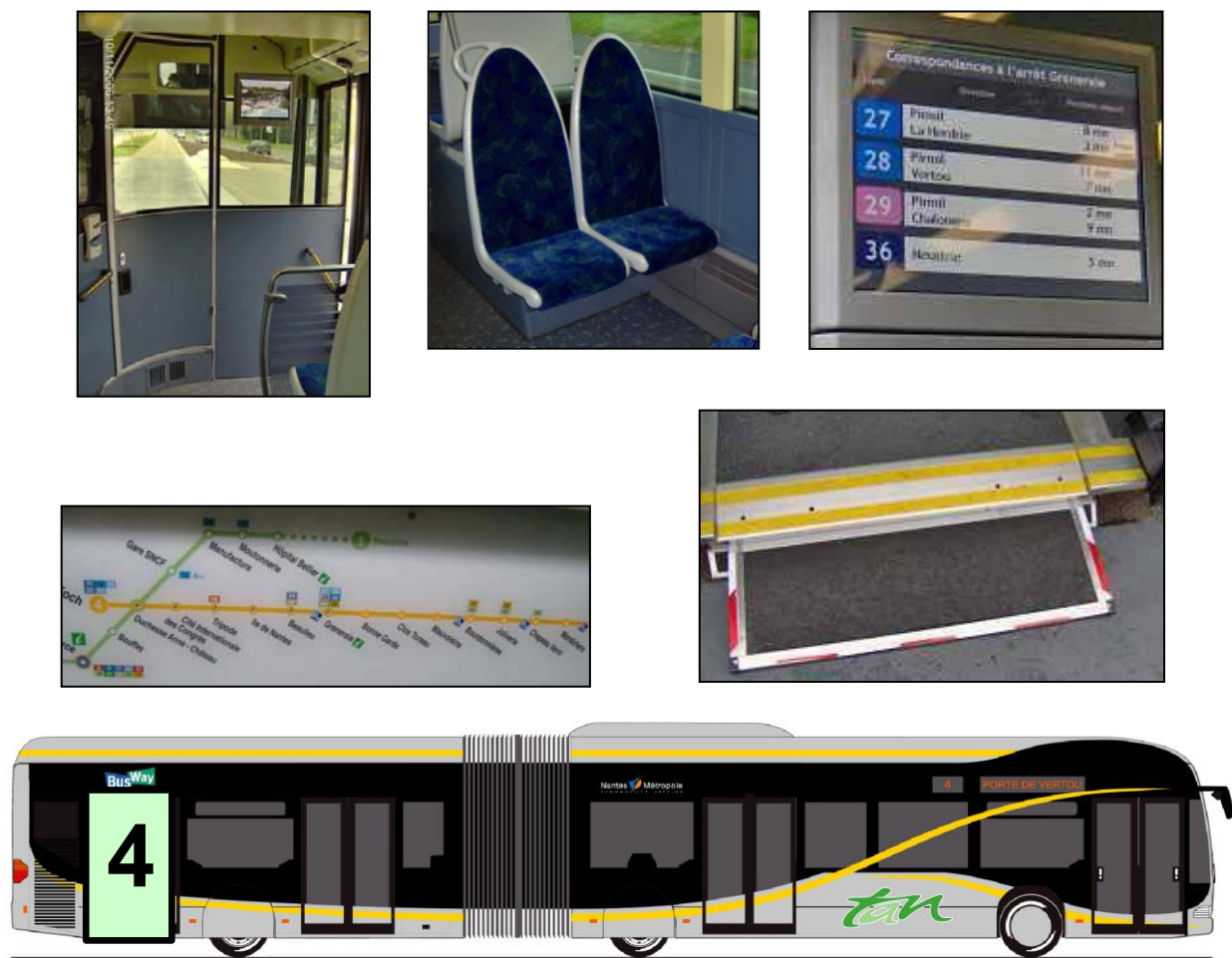
Figure 36: the Mercedes Citaro, adapted to incorporate typical tram-style components (source: Nantes Métropole)
