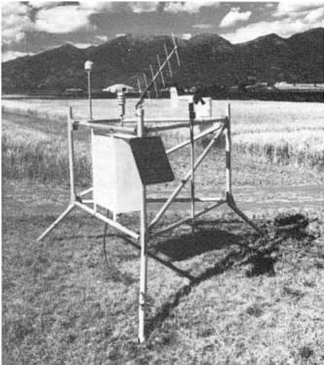
Figure 9-17.—Weather station and satellite platform.
