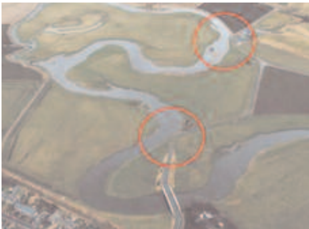
Figure 8: River migration affected by roads and river crossings (photo courtesy of Aberdeenshire Council)
