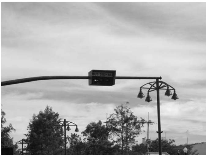
Figure 5-2. Orlando LYMMO's bus signal.
