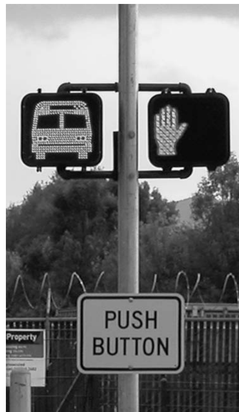
Figure 5-6. Bus-activated warning sign (black with orange symbol) for pedestrian midblock crossings of Orange Line busway, Los Angeles.
