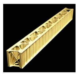
Deck Truss A bridge whose roadway is supported from beneath by a truss.
