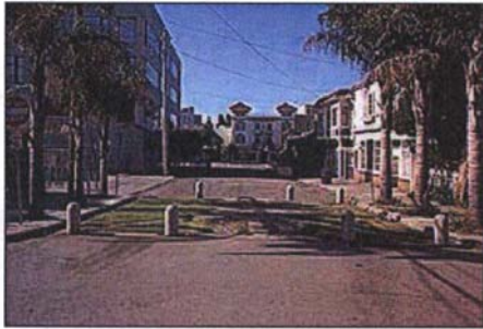
Berkeley, CA - This closure features removable bollards to prevent unauthorized motor vehicles from crossing, while allowing bicycles to pass along the narrow opening in the center.
