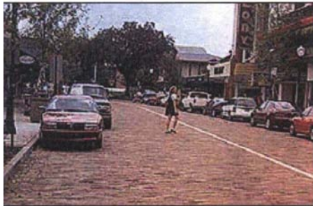
Winter Park, FL - This is a street with textured pavement and parallel parking.
