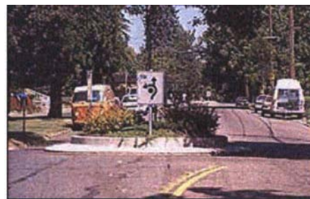
Seattle, WA - This traffic circle is located at a T-intersection, as indicated by the sign. A truck apron is included that allows trucks to make a left-turn, while passenger vehicles are discouraged from using the truck apron by the short lip at its edge.
