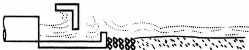
Impact Energy Dissipator
