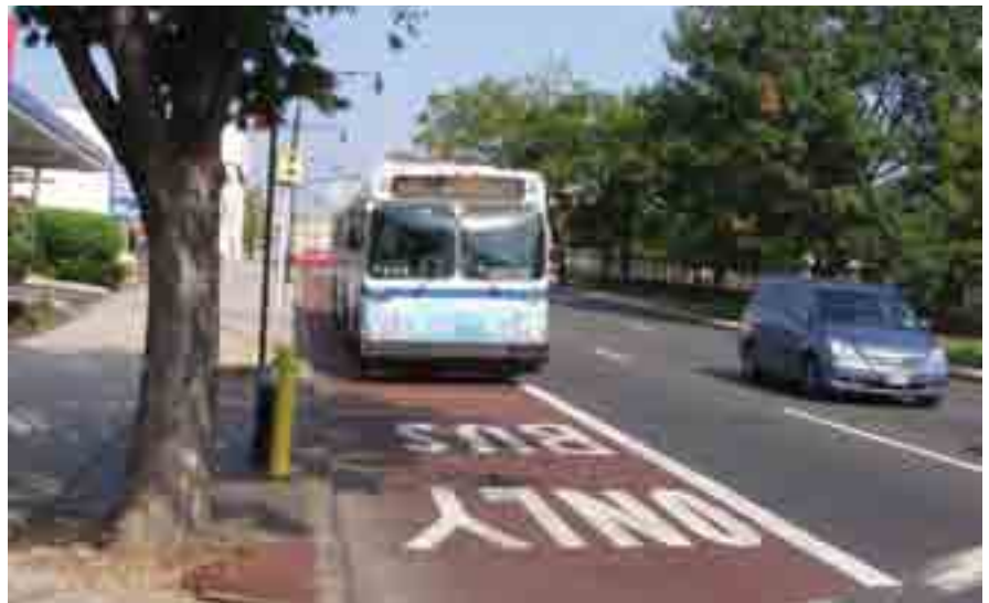
Red, curb-aligned, bus lane: East Fordham Road, The Bronx
