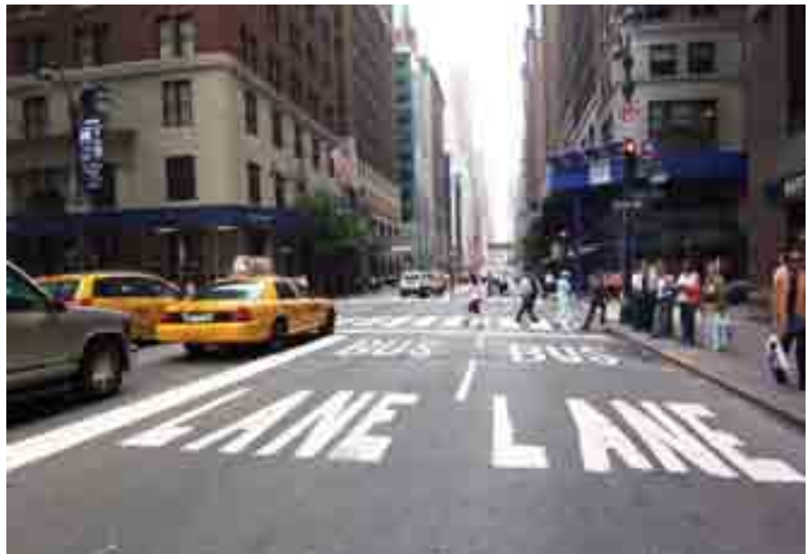
Curb-aligned double bus lane: Madison Avenue, Manhattan
