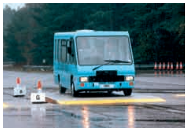
Fig. 2.1 Bus trials over flat-top humps
