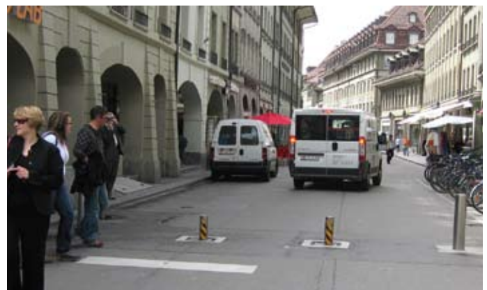
Figure 35. Retractable bollards provide access to pedestrian streets for authorized users in Bern, Switzerland.
