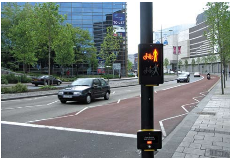
Figure 10. Near-side pedestrian signal with confirmation light in Bristol, United Kingdom.
