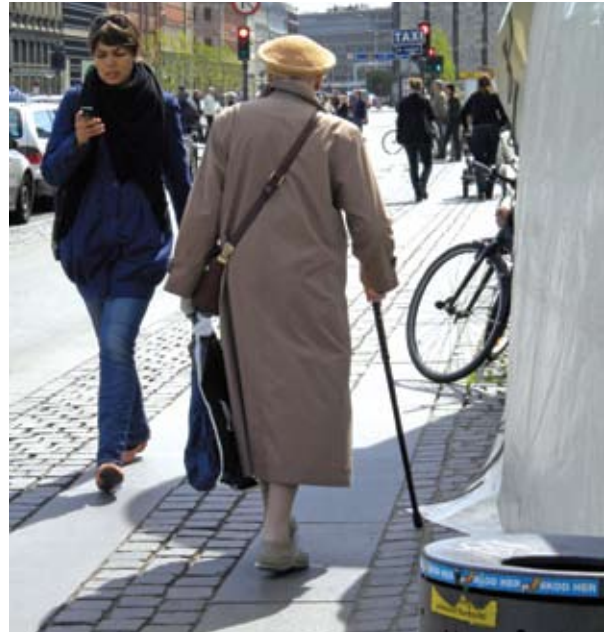
Figure 17. Smooth, accessible path on cobblestone sidewalk in Copenhagen, Denmark.
