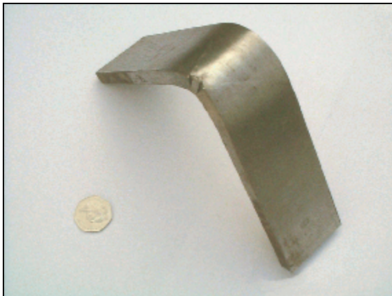
Bend test (note opening of root defect)
