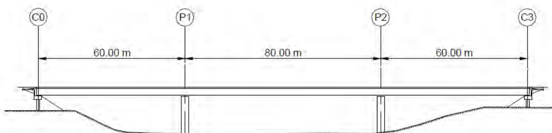
Fig. 3.2 Example of a three-span steel-concrete composite bridge
