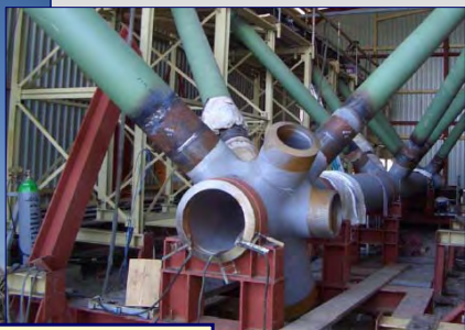
steel trusses with hollow sections and cast iron nodes
