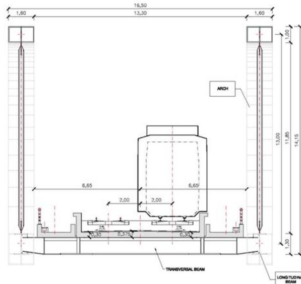
**Fig. 18:** Elevation and cross section of the Viaduct.
