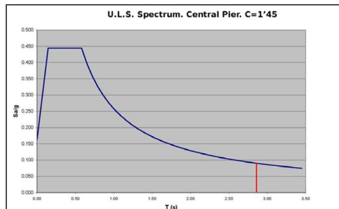
**Fig. 11:** Reduction of the seismic force for a longitudinal seismic action.
