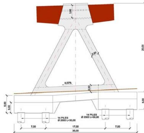
**Fig. 9:** Central pier elevation.
