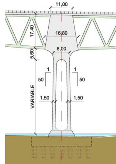
**Fig. 14:** View of the two inner piers P-6&P-7    **Fig. 15:** View of the two outer piers P5&P-8
