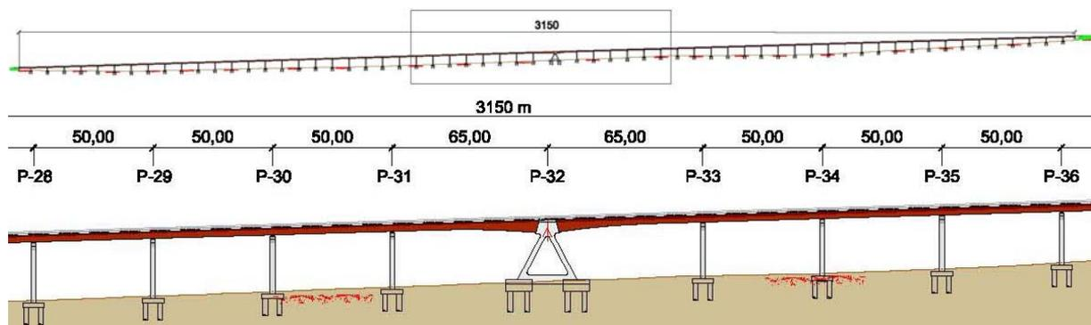
**Fig. 6:** Elevation view of “Archidona” Viaduct.
