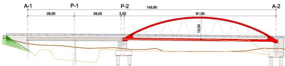
Fig. 17: Elevation and cross section of the Viaduct.
