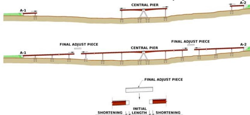
**Fig. 10:** Shrinkage deformation reduction by adjustment of erection process.
