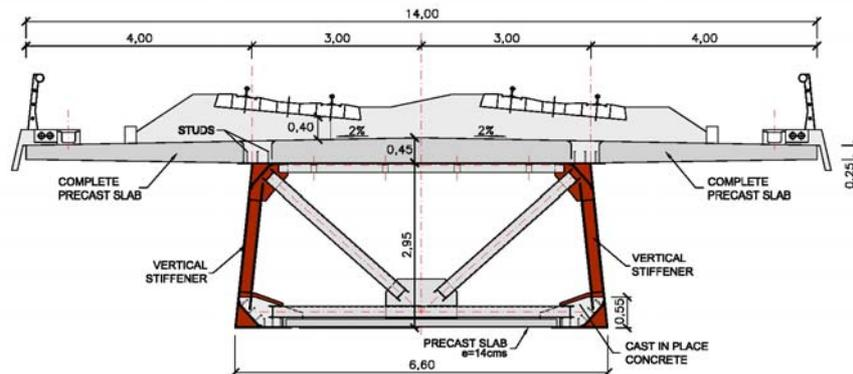
**Fig. 7:** Sagging cross-section
