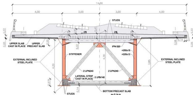
**Fig. 2:** Mid-span bending cross section
