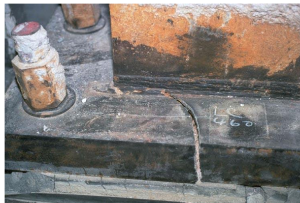
Fig. 1-12. Fractura en una placa de base de columna de una estructura de pórtico arriostrado (Earthquake Engineering Research Institute, Slides on the January 17, 1994, Northridge Earthquake, Set I: An Overview).
