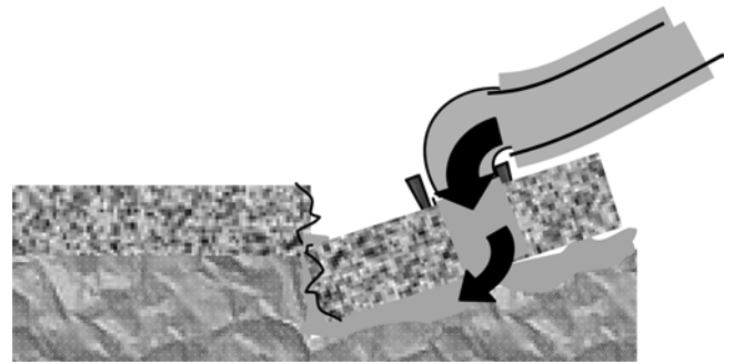
Fig. 5—Pumping of the slabjacking grout in the drilled hole showing grout flow resulting in slab displacement.
