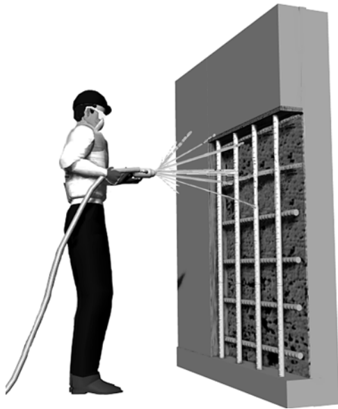
Fig. 3—Presaturate prepared surface with water.
