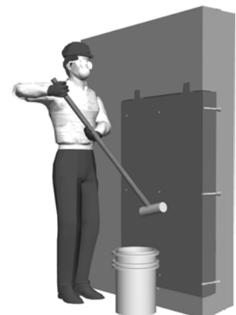
Fig. 4—Material placement: vertical application.
