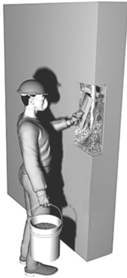
Fig. 8—Hand application of repair material.
