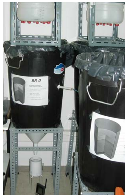
Figure 7. Laboratory equipment to evaluate the pervious pavement functionality.
