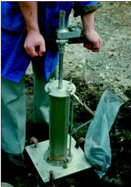
▲ 4 - Compaction inspection with a membrane densimeter...
