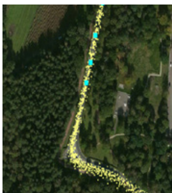
Illustration 24. - Braking Centroids for Various Entering Speeds (from top to bottom: 70km/h, 60km/h, 50km/h, and 40km/h)
