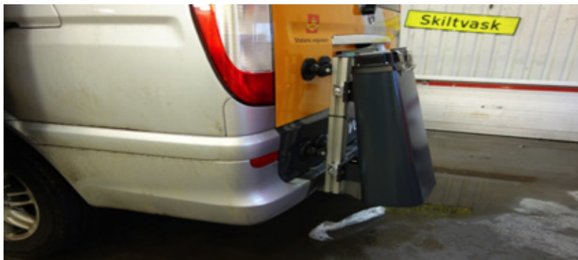
Illustration 16 - Marwis optical sensor from Lufft to be tested in the ROSTMOS project; will be compared with Teconer RCM411 and MetRoad Mobile, from MetSense.
