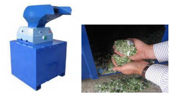
*Fig. 4.3. (a)* GLASSVAC's GP3 Cube and (b) view of the final glass waste after the implosion process.
