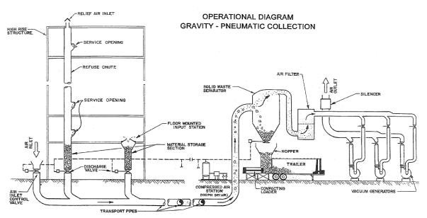
Fig. 3.1. Schematic diagram of the Roosevelt island AVAC operation.
