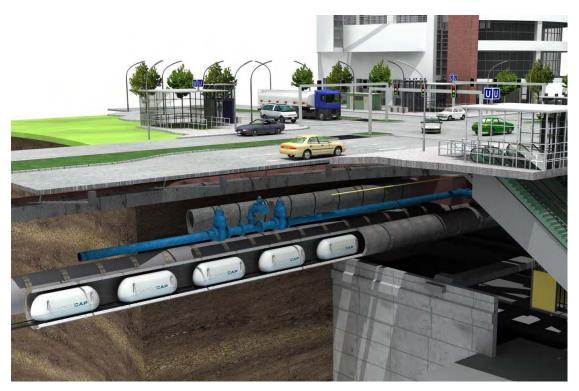
Fig. 4.1. Underground freight transportation using capsules (source: Cargocap GmbH. 2012).
