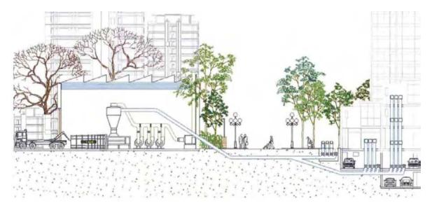
Fig. 3.8. Schematic view of the automated waste collection system operated at 2004 Forum area.
