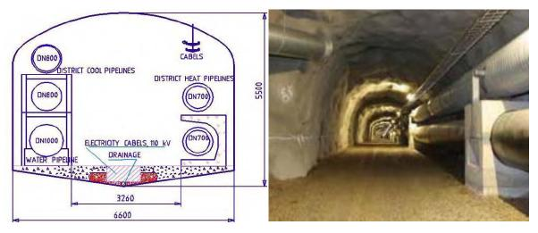
*Fig.* 4.2. (a) *Indicative sketch and* (b) *inside view of multi-purpose utility tunnel.*
