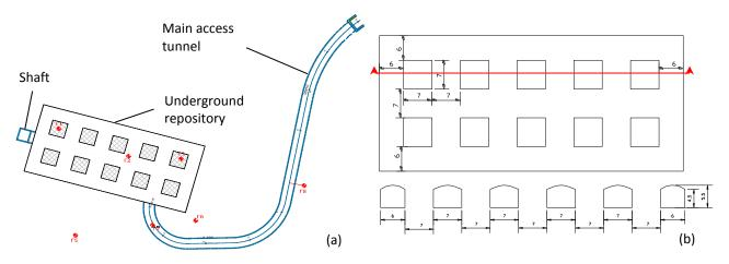
*Fig. 3.13.* LTCP underground hazardous waste repository (a) general layout of the underground complex, (b) detailed plan of the room and pillar arrangement followed at the main storage area.
