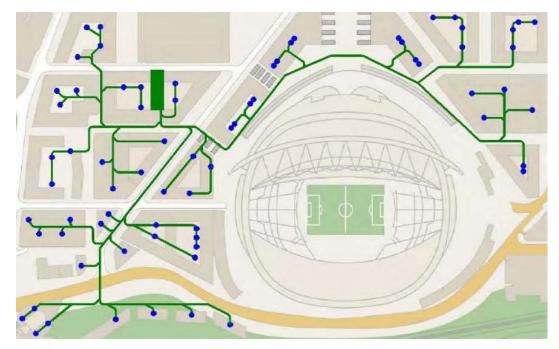
*Fig. 3.4. Schematic drawing of inlet points and the underground pipe network for the AVAC development in Wembley city.*
