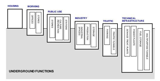
*Fig. 1.1. Feasible depths for the development of underground use types in the urban structure (Ronka et al., 1998).*
