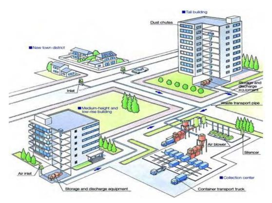
Fig. 2.9. General schematic view of the equipment and the layout used for the AVAC system.
