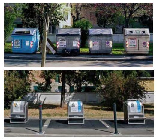
*Fig. 2.3. Above ground and underground waste collection systems (source: Ecologia Soluzione Ambiente SpA, 2012).*
