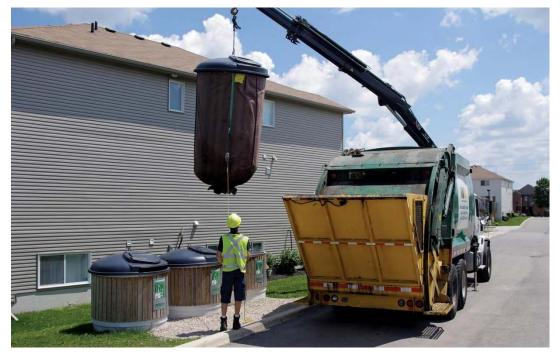
Fig. 2.5. Waste collection process in Molok type underground waste containers.
