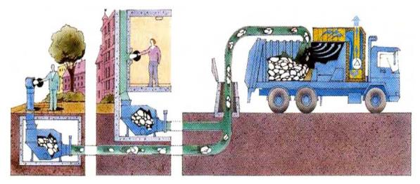
*Fig. 2.10. Mobile vacuum units facilitating the handling of wastes from underground waste collection points.*
