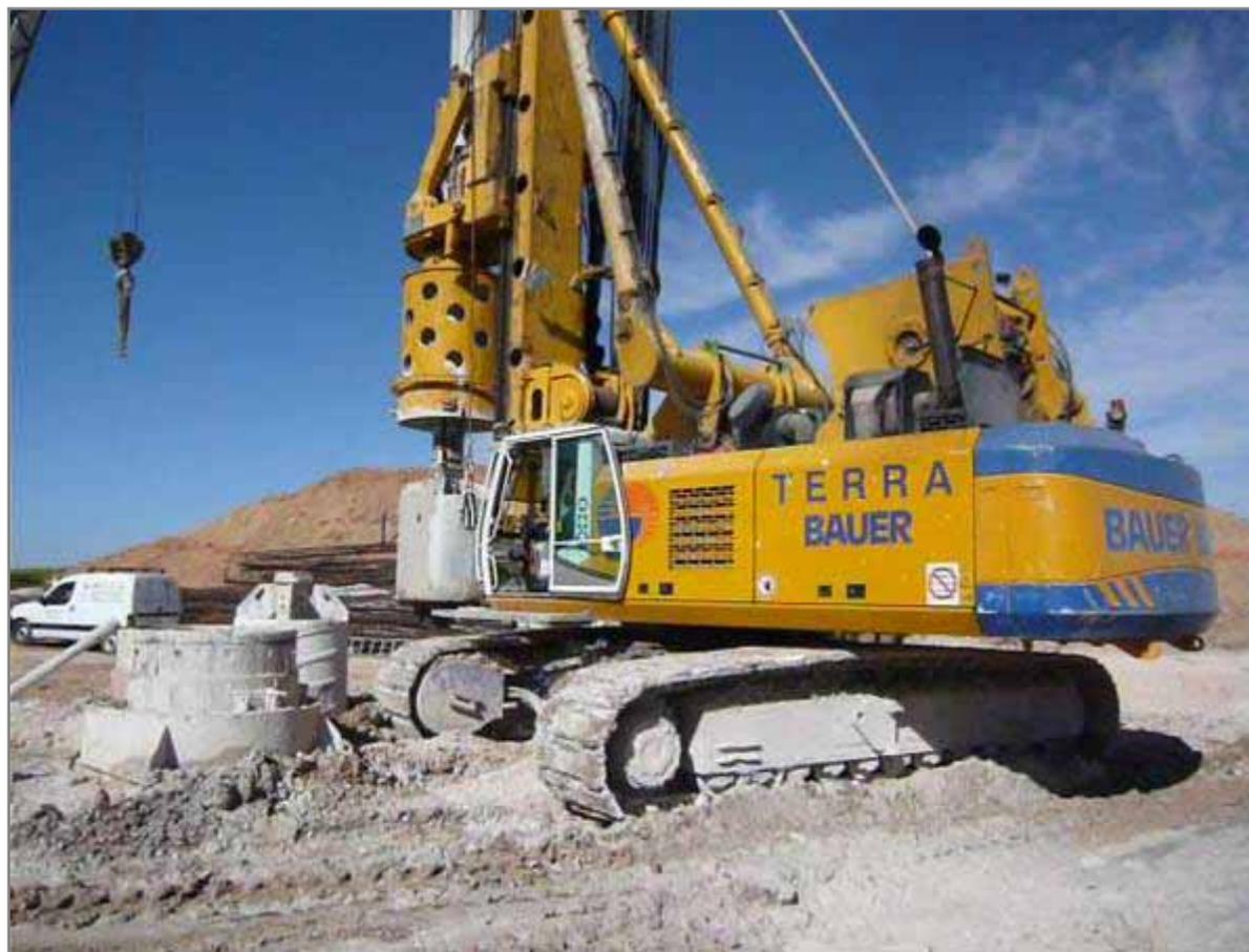
EQUIPOS DISEÑADOS PARA PERFORAR TERRENOS “BLANDOS”
