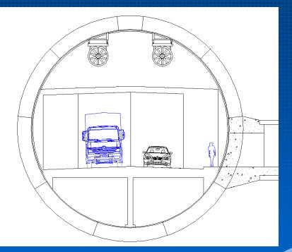
'Normal' section showing exhaust duct (upper, 28m<sup>2</sup>) & fresh air supply duct (below roadway, 26m<sup>2</sup>)
